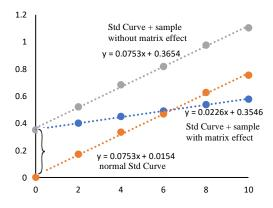
Difference between 0 Standards is 0.35. Slope in the presence of sample is 0.226 OD/nmole. Amount of analyte in sample with matrix effect = 0.35 OD / 0.226 OD / nmole = 1.55 nmole
